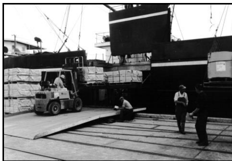
In the beginning, sideport operations on "Shansi". 1 ton pallets.
